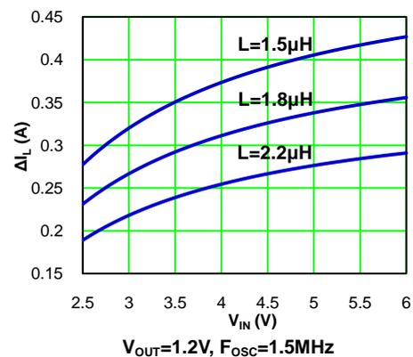
A good compromise value between size and efficiency is to set the peak-to-peak inductor ripple current  $\Delta I_L$  equal to 30% of the maximum load current. But setting the peak-to-peak inductor ripple current  $\Delta I_L$  between 20%~50% of the maximum load current is also acceptable. Then the inductance can be calculated with the following equation:
